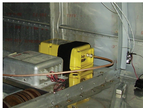
Panel unit (top) and main unit (bottom) of Artex ME-406 ELT installation in 891JH
